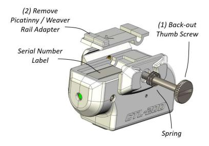
Note: If you fully remove the thumb screw, take care to retain the spring.
